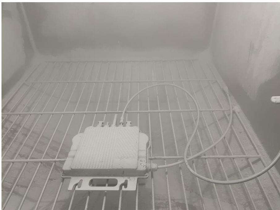
Test setup of IP6X
