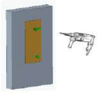
13. Install screws on the positioned hole 14. Install the bracket
