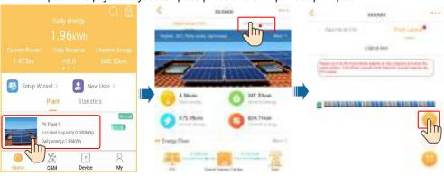
2. Log in to https://intl.fusionsolar.huawei.com to access the WebUI of the FusionSolar Smart PV Management System. On the **Homepage** page, click the plant name to go to the plant page. Select **Plant layout**. Choose ① > **Generate with AI**, and create a physical layout as prompted. You can also manually create a physical location layout.
