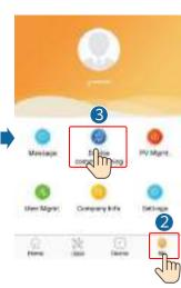
2. Connect to the solar inverter WLAN and log in as **installer** to access the device commissioning screen.
