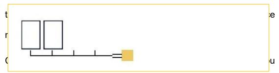
can choose install the micro-inverter at left or right side of the panels.
