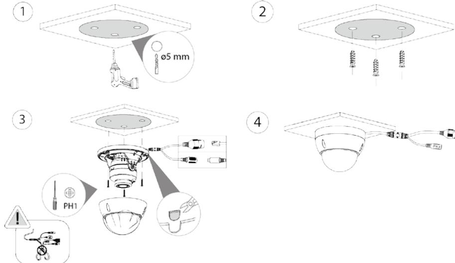
Figure 3-8 Cable going through the mounting surface
